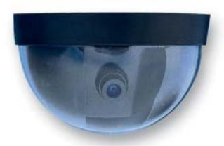
Our 1/4" color CCD dome camera with smoked housing can be mounted on the ceiling and offers unobtrusive surveillance with its' black housing. It can be rotated a full 360 degrees and tilted +/- 90 degrees for maximum viewing selection. It features 1.0 lux sensitivity with 420 line resolution and a 3.6mm wide angle lens with built-in electronic shutter. A 12V DC power supply is included.
